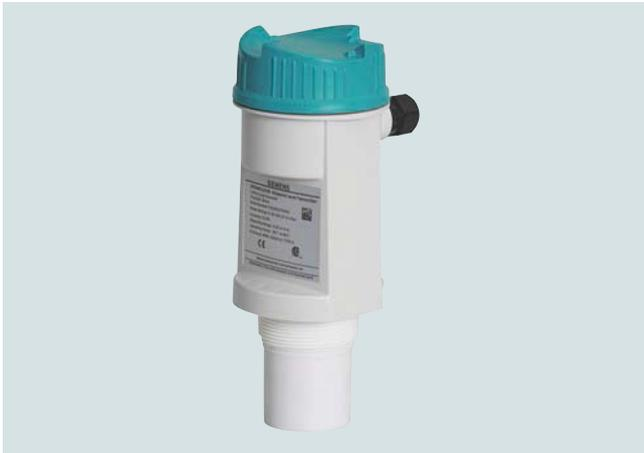
SITRANS LU180 is a short-range integrated ultrasonic level transmitter. It is intrinsically safe (ATEX, CSA, FM, IECEx, NEPSI), 2 wire, 4 to 20 mA loop powered, ideal for liquids, slurries, and bulk materials in open or closed vessels to 5 meters (16.4 feet).
