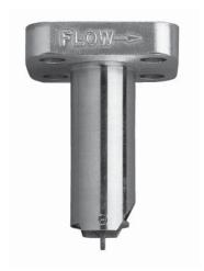
The Signet 525 Metalex Paddlewheel Flow Sensor combines stainless steel construction with insertion paddlewheel technology. The result is a highly reliable sensor suitable for operation at extreme pressures and temperatures. The Tungsten Carbide shaft and carbon fiber reinforced PTFE bearing provides excellent wear resistance for extended service.
